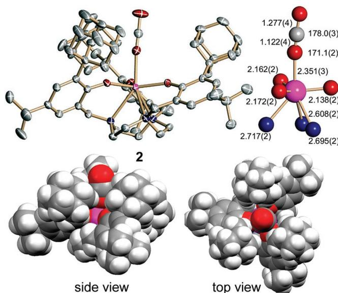
Fig. 1. ORTEP (Oak Ridge thermal ellipsoid plot) of uranium CO<sub>2</sub> complex **2** and in crystals of **2** · 2.5 Et<sub>2</sub>O (top left) with core structure and metric parameters in angstroms and degrees (top right) and space-filling representations (bottom). Uranium, magenta; nitrogen, blue; oxygen, red; carbon, gray.
